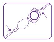
Connect water bag tube to the pump.
