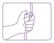
Open the valve and compress pump so that tube and pump fills with water (turn pump other way up to fill and remove air). Then close the valve.
